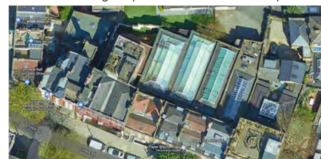
Cross Street Warehouse backs suitable for triple/quad roof lights and high levels of roof insulation
